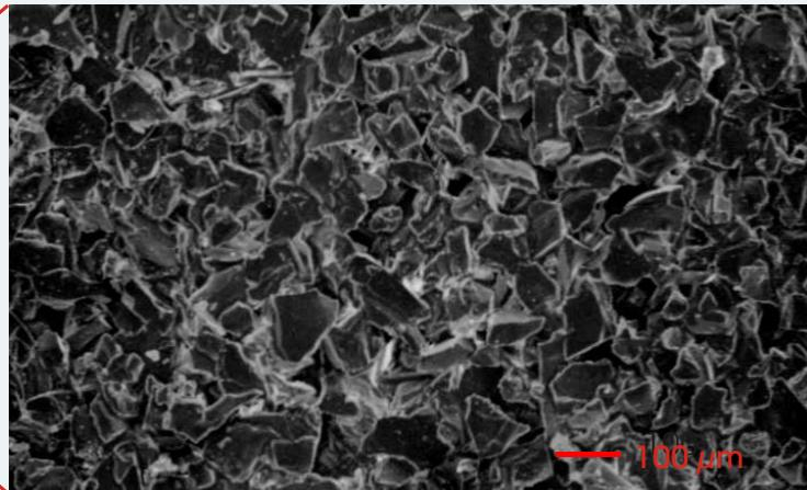
Porous ceramic 37% open, 20  $\mu\text{m}$  pore size
